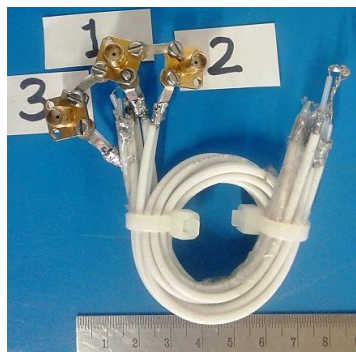
FIG. 4: Photograph of the proposed miniaturized 1: 4 UWPD the coaxial cables (where 1, 2, and 3 indicates the port numbers)
